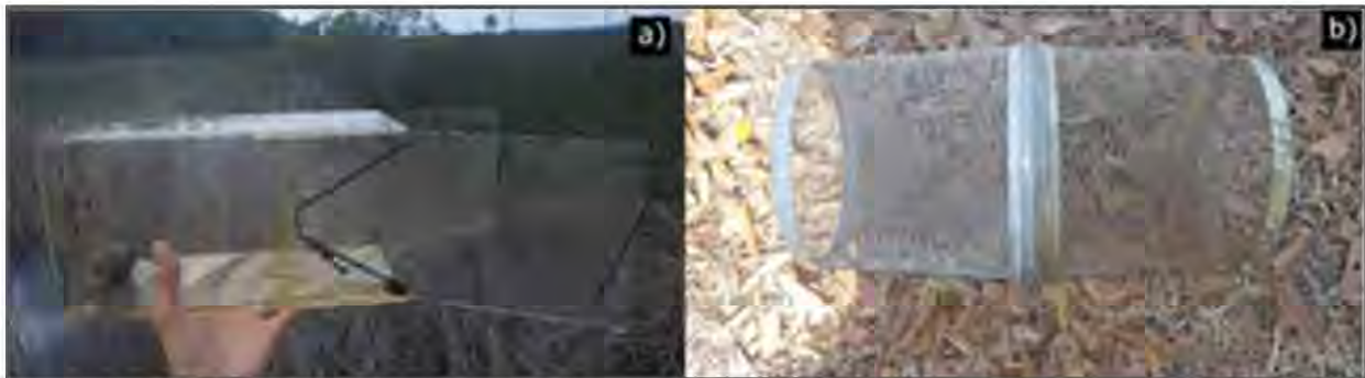
Sampling gears used to sample saltmarsh topminnows: a) Breder Trap, b) Gee minnow trap.
