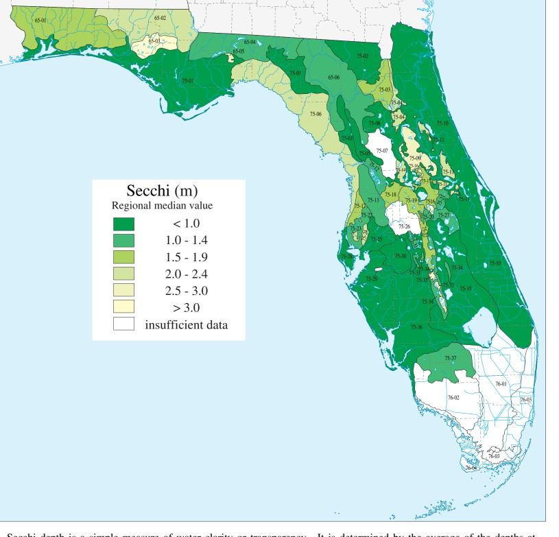
Secchi depth is a simple measure of water clarity or transparency. It is determined by the average of the depths at which a black and white disk disappears and reappears when viewed from the water's surface. The secchi depth is dependent upon the turbidity, color, and total suspended solids in the water, among other factors. The low-color lakes of the upland ridges (65-03, 75-04, 75-09, 75-15, 75-20, and 75-33) generally have the greatest secchi depths.
