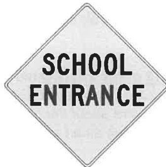
Figure 15-1 School Entrance Warning Sign (FTP 33-06)
