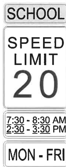
Figure 15-10 School Speed Zone Time Enforcement Sign
