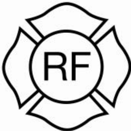
Light-frame "Floor & Roof"
